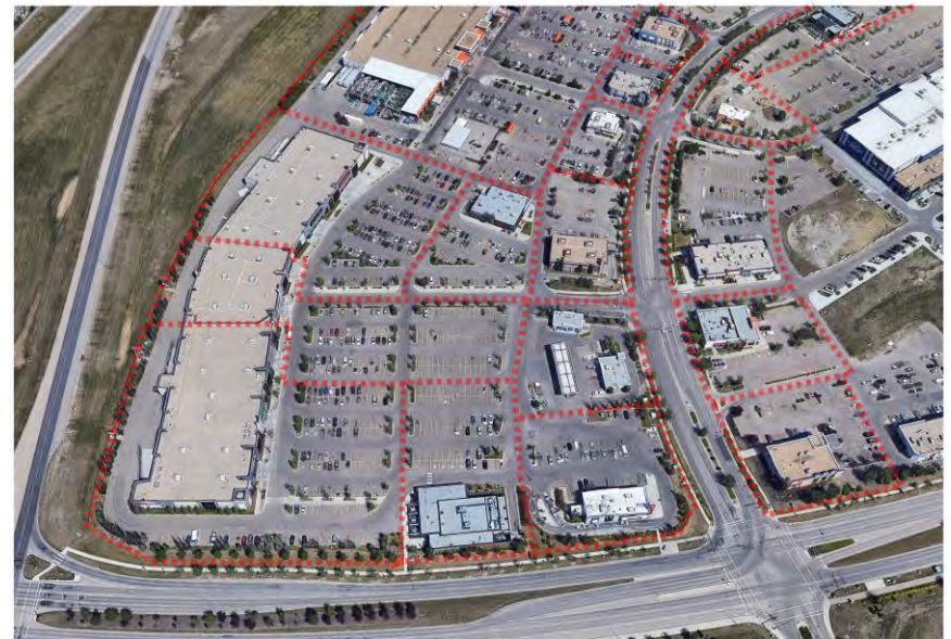
Shared parking with individual development limits for each building or phase. This allows parking and pedestrian movement to be shared but development requirements for each site can be met individually.
